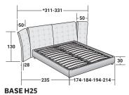
ADJUSTABLE SLATTED BASE ELECTRICALLY POWERED ADJUSTABLE SLATS
